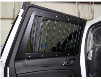
Installation Complete. **To clean windows, unscrew guard from upper bracket.**
