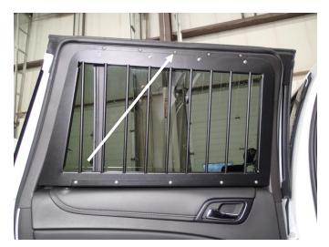
Mark and drill five (5) 5/32" holes in door / window frame for upper bracket. Screw upper bracket to door frame with # 10 x 1/2" flat head sheet metal screws. Tighten hardware
