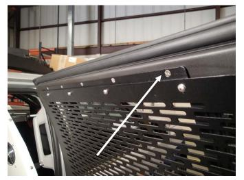
Mark and drill 5/32" holes in door / window frame for upper bracket. Screw upper bracket to door frame with # 10 x 1/2" flat head sheet metal screws. Tighten hardware
