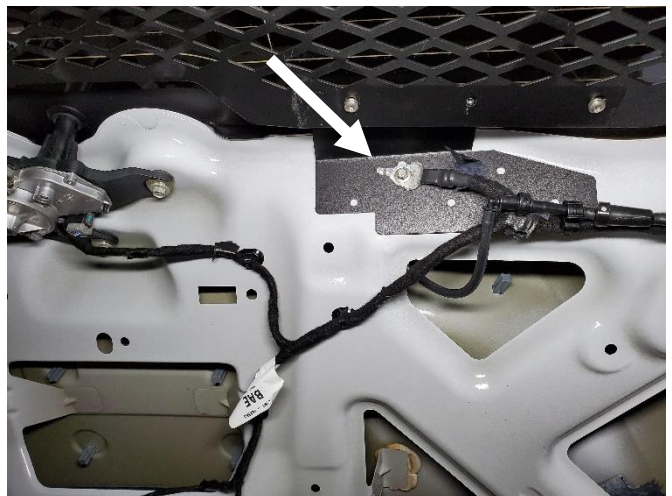
Line up to previously removed OEM fasteners. Re-install fasteners in slotted holes in bracket and tighten.
