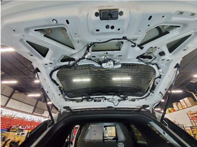
Carefully remove OEM trim from rear hatch
