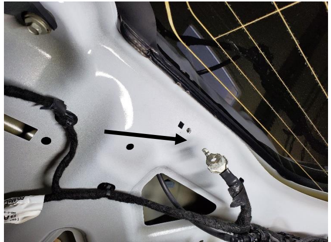
Temporarily remove ground bolt from driver side of trim panel. (5/16 socket)
