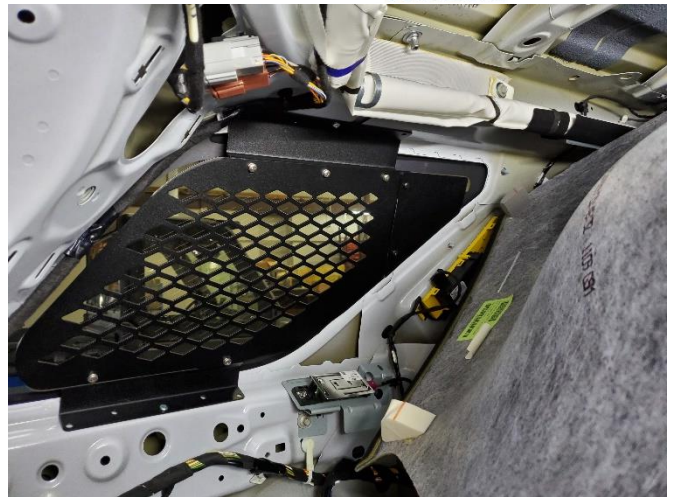
Place window screen or bars into window opening. Center window guard between black tint on glass.
