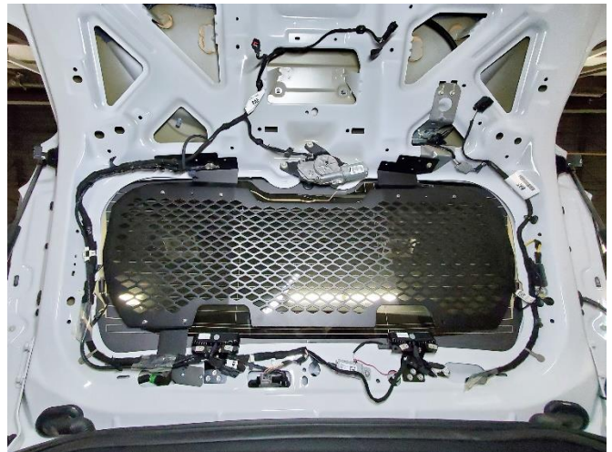
Attach mounting brackets to rear window screen and hold up to interior window frame.
