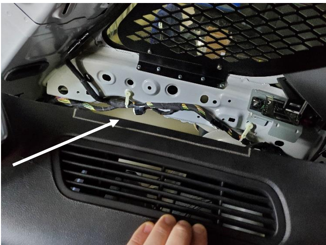
Notch plastic as needed and reinstall all trim. Notching headliner not required. Repeat for other side
