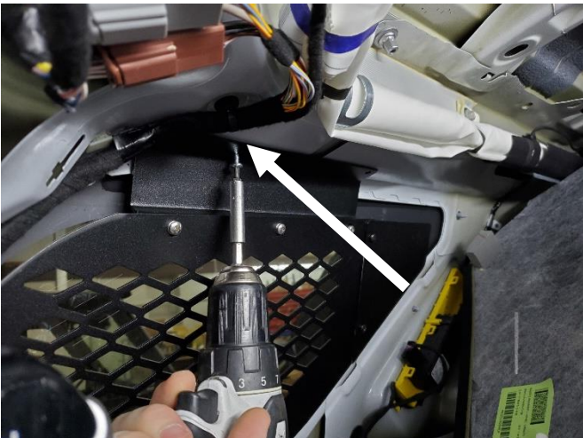
Mount brackets steel window frame with #10 x 1/2" TEK screws.
