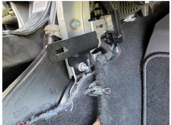
Install Passenger side forward mounting bracket.
