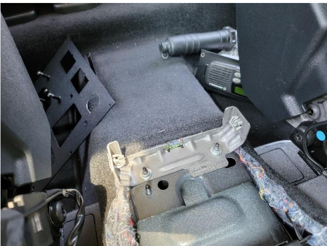
Remove OEM rear mounting bracket from floor of vehicle.
