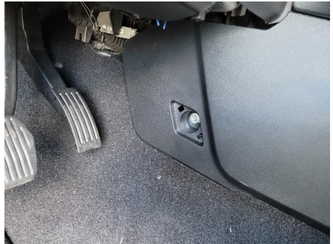
Remove cover from lower driver side panel. Unbolt the 13mm OEM fastener and set aside.
