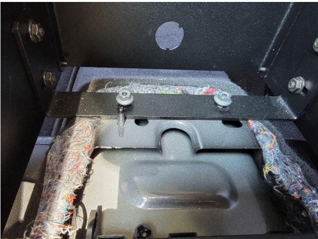
Attach rear-mounting bracket to floor studs at rear of console. Tighten using OEM nuts.
