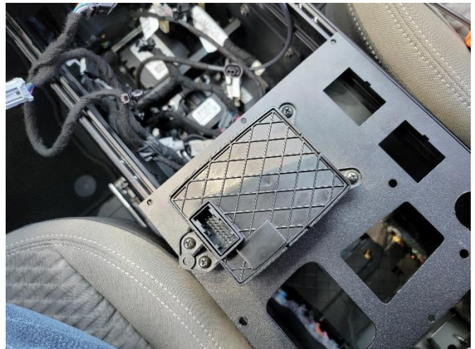
Install shifter into console plate with supplied 10-32 x 1/2" machine screws.
