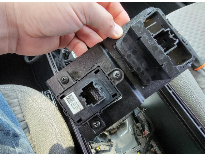
Snap Mode control into Mode switch bracket. Attach emergency brake switch using 10-32 x 1/2" screws.
