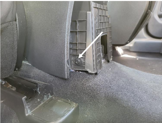
Unsnap rear section of console and remove (2) 10mm head fasteners. Remove OEM console from vehicle.
