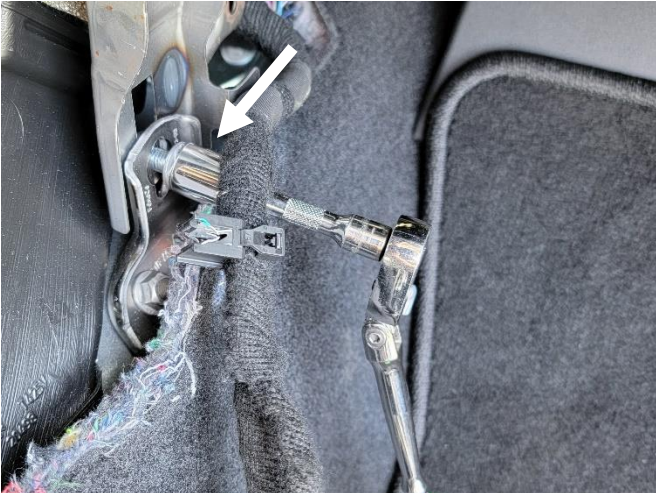
Remove 13mm bolt from brace at front of vehicle on passenger side.
