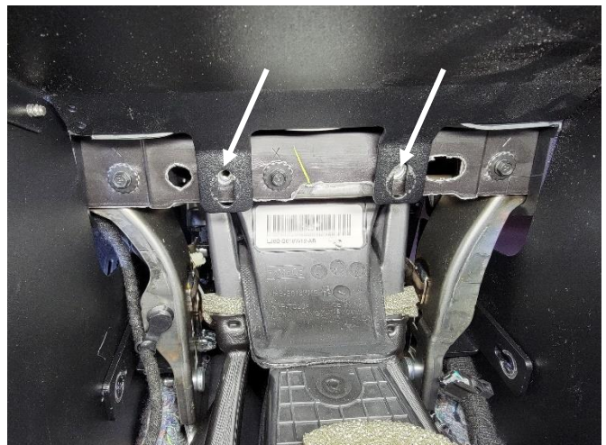
The front of the console should be lined up with inserts for OEM fasteners.
