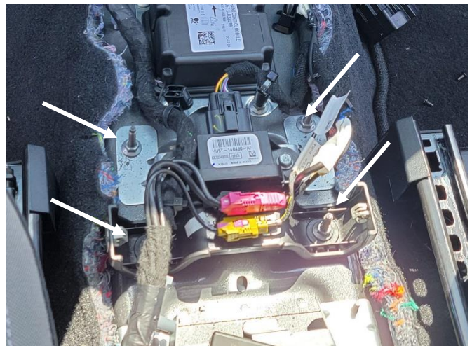
Loosen (4) 10mm head nuts from mid-section of transmission hump.
