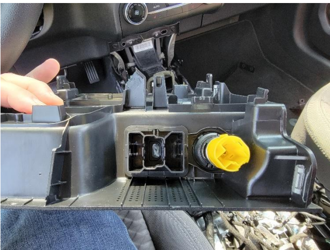
Remove USB plate and 12v socket from forward console plate.
