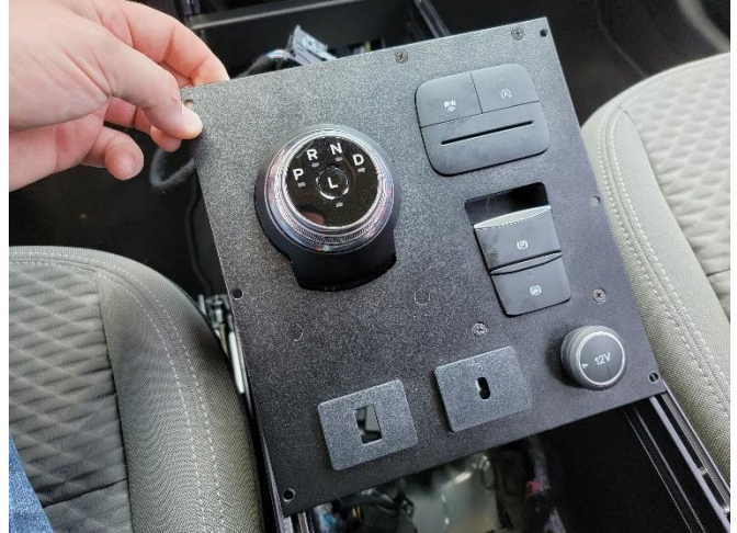
Verify all modules are attached, snug and no buttons are binding. O-ring supplied is used as spacer for USB module to be a tighter fit.
