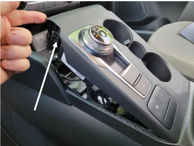
Lift up center shifter plate by gently prying from the front and lifting up.
