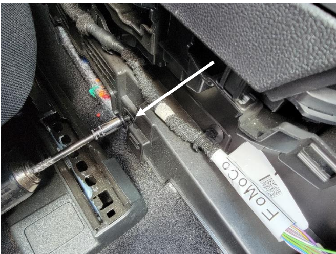
Remove side trim panels from OEM console. Remove 10mm head fasteners from lower side of OEM console.
