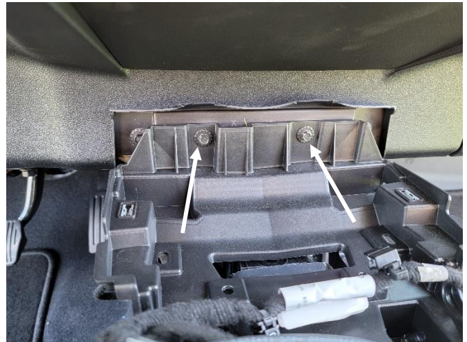
Remove (2) 8mm head fasteners from front section of console.
