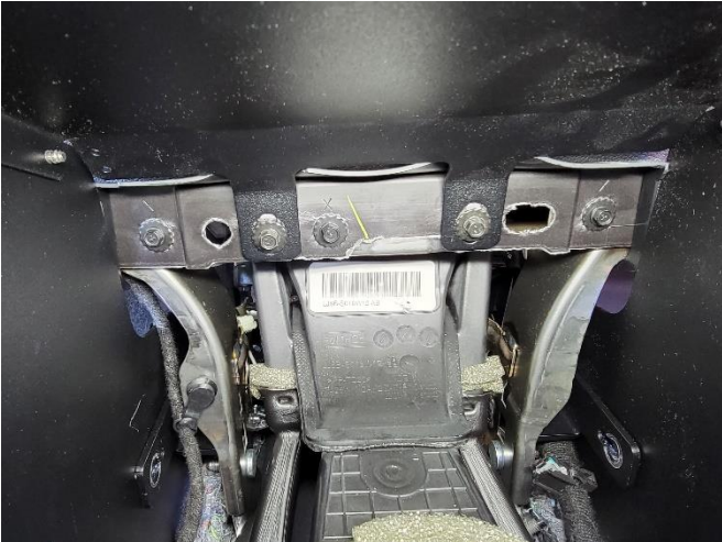
Reinstall previously removed OEM fasteners through front of console.
