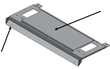
Place base bracket 26460 into vehicle and attach to OEM floor holes using previously removed third row seat OEM bolts or provided M10x1.50x45 bolts and washers. Two (2) 0.77" spacers are used for front bolts only. Attach electronics tray to base bracket with six (6) Torx screws.
