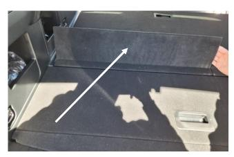
Prior to re-installing OEM rear storage bin, the hinged flaps must be cut off in order to fit.
