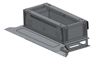
The rear hinge cover that comes with K9-F27-1 must be replaced with cover included in the SBX-5016 kit. Use 10/32 nuts to attach cover to hinge studs on K9 insert back wall. Attach cover to storage box mount top bracket using four (4) 1/4"X 3/4" screws and serrated flange nuts.
