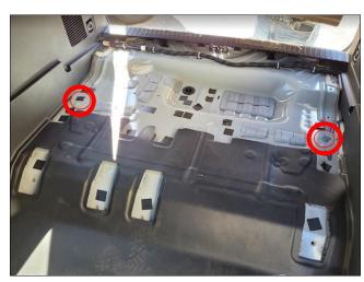
For a vehicle with no third row seat, remove tape over two circled holes and tap with M10x1.5 thread.
