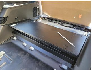
Attach mount plate to risers with 10-32 X 1/2 Phillips flat head machine screws and nuts.
