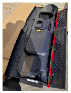
Detach springs from OEM rear storage bin flaps and cut flaps approximately at hinge point shown by the red line. Reinstall rear storage bin.
