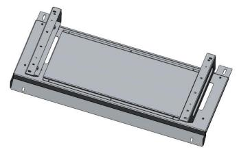
Attach riser brackets to base with 5/16" X 3/4" Hex head bolts, lock washers and flat washers.
