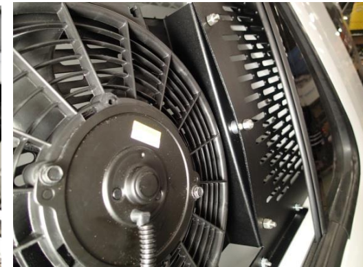
Attach optional 10" fan and fan mount to window guard with 1/4" hardware and spacers as per the instructions provided in the optional K9-A-104 kit.
