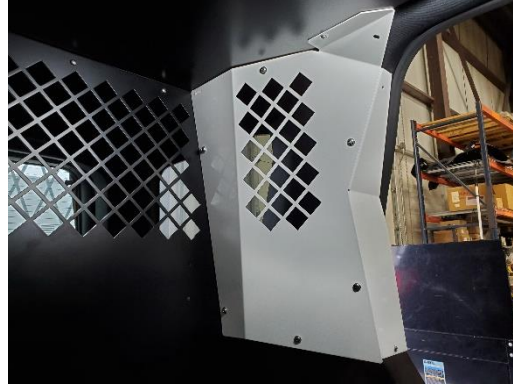
Attach upper side trim panel to rear wall lower corner trim panel and upper forward side trim panel using 1/4" x 3/4" Phillips bolts and washers.
