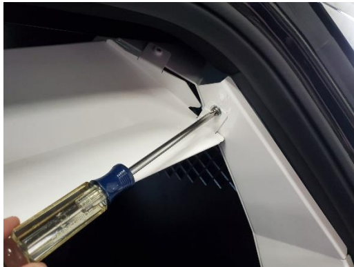
Attach upper ceiling trim panel to upper side trim panel using 1/4" x 3/4" Phillips bolt and washer.
