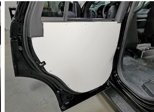
Attach the K9 door panel using the supplied #10 x 1/2" sheet metal screws.
