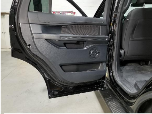
Remove rear passenger door panels first.
