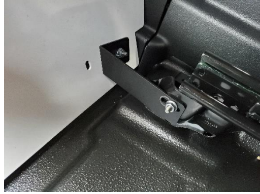
Attach lower support bracket to OEM hole in driver seat base and to bulkhead using (2) 1/4" x 3/4" carriage bolts and nuts.
