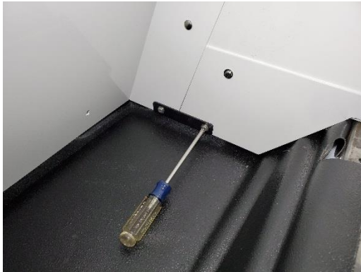
Attach lower divider filler support bracket using (2) 1/4" x 3/4" Phillips head bolts and washers.
