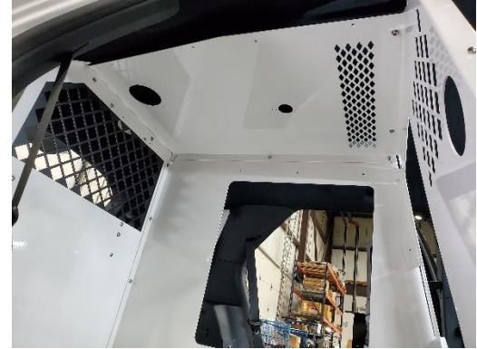
Place ceiling on top of front and rear bulkheads. Loosely attach ceiling to rear bulkhead with 1/4" x 3/4" pan head Phillips bolts and flat washers.
