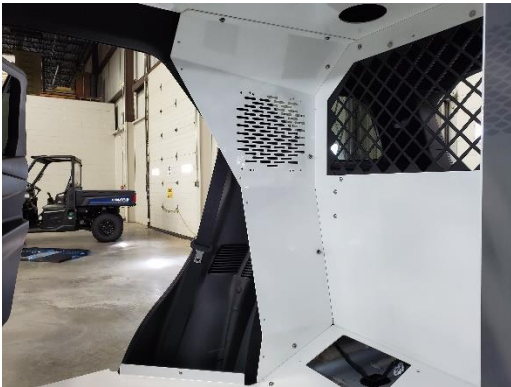
Attach K9 side wall to kit and using 1/4" x 3/4" pan head Phillips bolts and flat washers.
