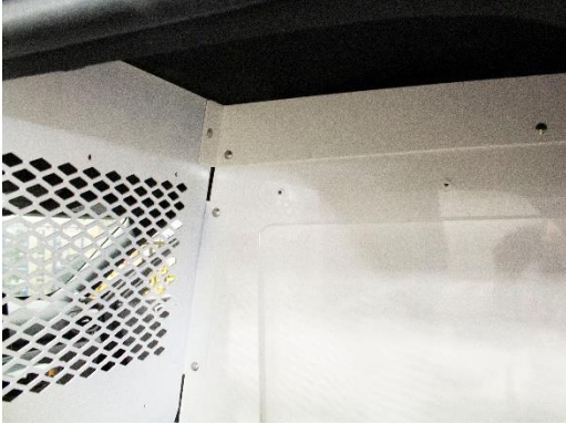
Attach upper trim panel to center divider and front bulkhead using (3) 1/4" x 3/4" carriage bolts and serrated nuts.
