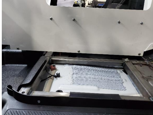
Attach divider to bulkheads using 1/4" x 3/4" carriage bolts, Phillips bolts, and washers.
