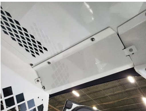
Attach K9 upper trim into kit using 1/4" x 3/4" pan head Phillips bolts and flat washers.
