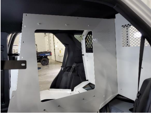
Place divider wall into vehicle and line up to passenger side front and rear bulkhead.
