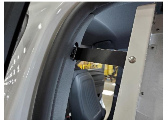
Attach partition to previously installed "B" pillar brackets using 1/4" x 3/4" carriage bolts and serrated nuts.
