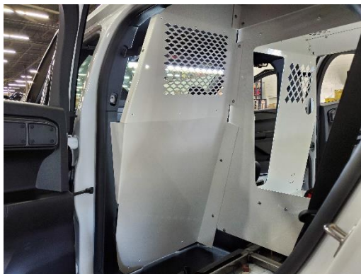
Place the prisoner partition into vehicle and attach using 1/4" x 3/4" carriage bolts and serrated nuts.
