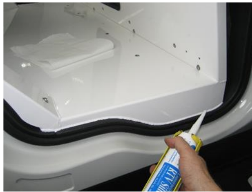
Neatly silicone / caulk the lower seams to shed water out of vehicle. Let silicone dry overnight prior to installing rubber mat
