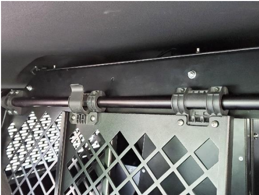
Confirm smooth slide and lock functionality of front egress door.
