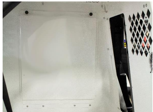
Install center emergency exit pass through door by placing on bottom support and securing at top studs using (2) 1/4" knobs.
