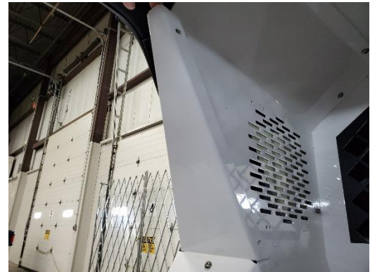
Attach K9 upper rear filler to kit using 1/4" x 3/4" pan head Phillips bolts and flat washers.
