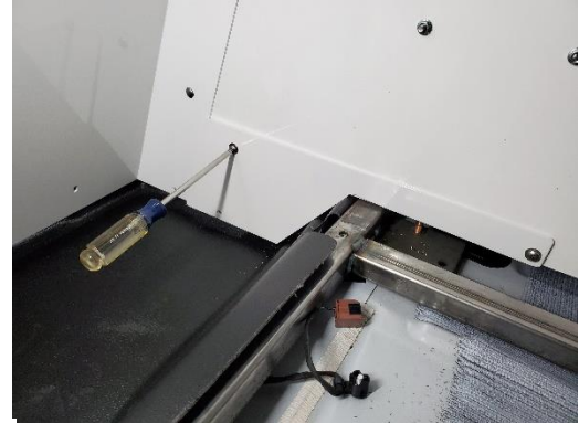
Attach lower filler to divider using 1/4" x 3/4" pan head Phillips bolts and washers.
