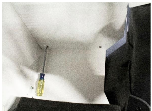
Install lower filler behind rear seat using (3) 1/4" x 3/4" pan head Phillips bolts and washers.
