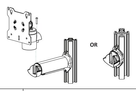
**Step 2:** Attach your VESA Monitor to the Double Pivot Mount using the 4x M4 x 10mm Phillip Screws as shown
