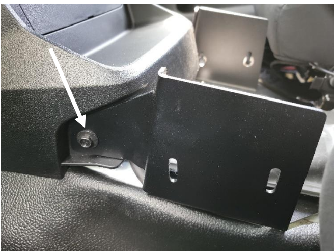
Line front of bracket up to center dash. Attach using previously removed 10mm head fasteners.
