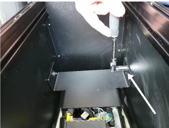
Attach rear of console to rear mounting bracket with 1/4" x 3/4" carriage bolts and serrated nuts.
