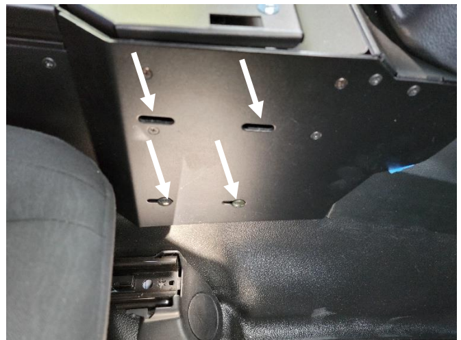
Attach passenger side of console to front mounting bracket with 1/4" x 3/4" carriage bolts and nuts.
