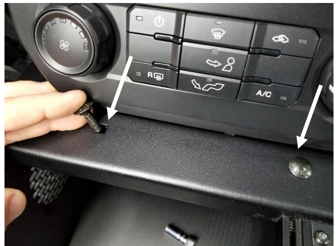
Attach front top console to mounting tabs with 1/4" x 3/4" carriage bolts and 1/4" serrated nuts.
