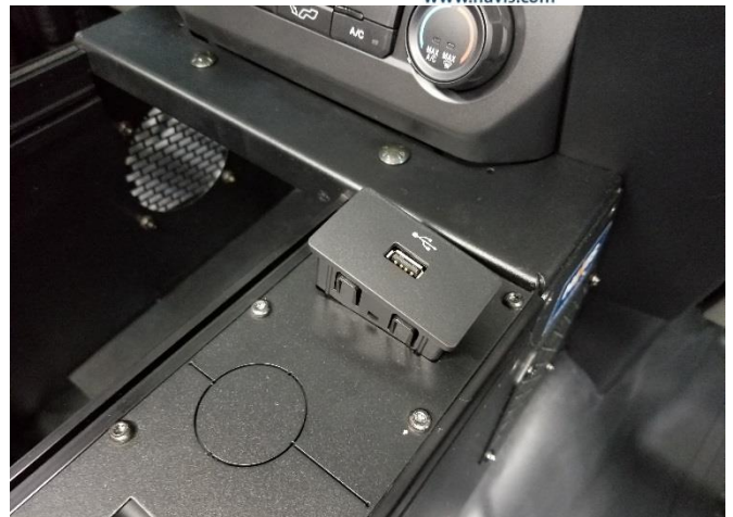
Install OEM AUX module into the console. Adaptor plate with #8 flat head screws provided for smaller Aux module. Blank plate provided if vehicle has no module.
