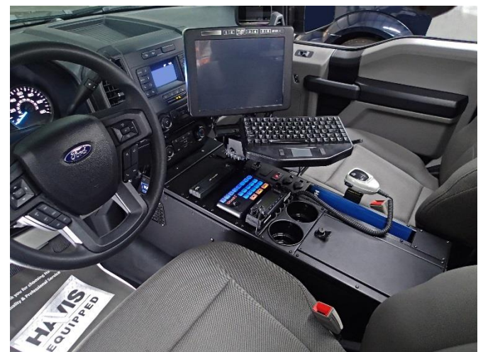
Console with computer installation complete
