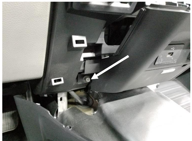
Remove (2) 10mm head fasteners from either side of storage pocket.
