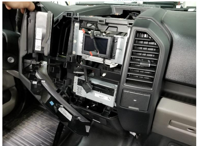
Remove the side vent trim on both sides of the radio.
