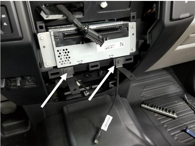
Install front mounting tabs using OEM hardware
