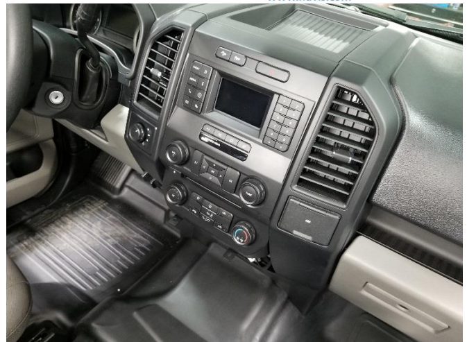
Reinstall previously removed center IP and upper storage tray.
