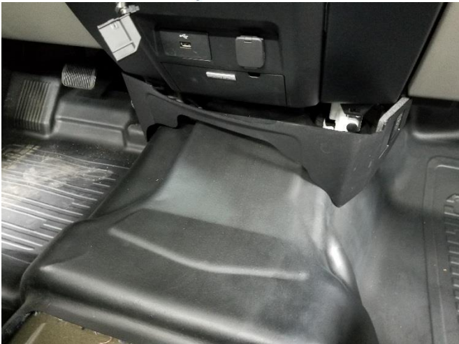
Starting on the passenger side, unclip and pull the lower dash cover trim off.
