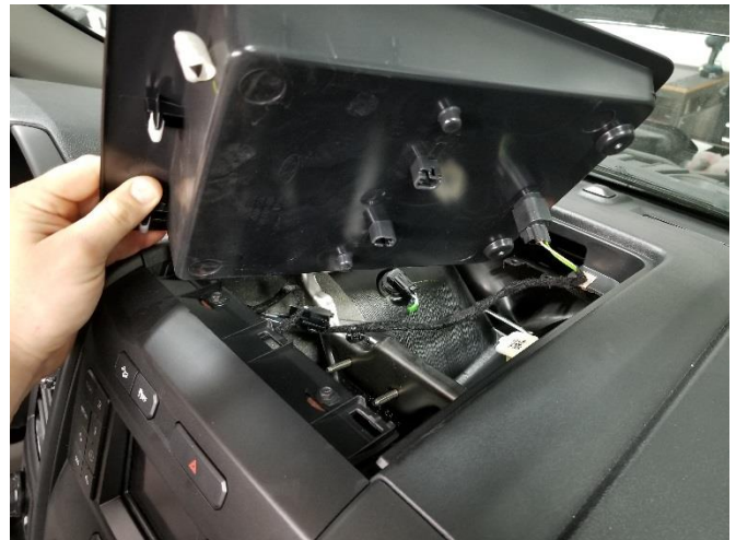
Unbolt upper storage tray from dash by removing (2) 7mm head fasteners
