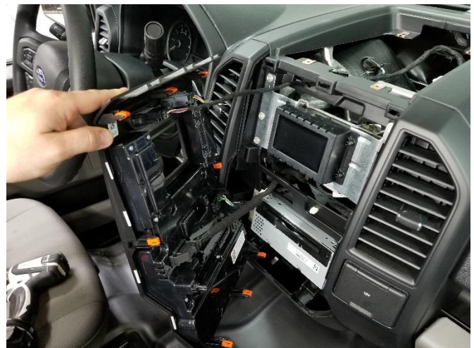
Gently remove the center instrument panel (IP). Unplug everything and set aside.
