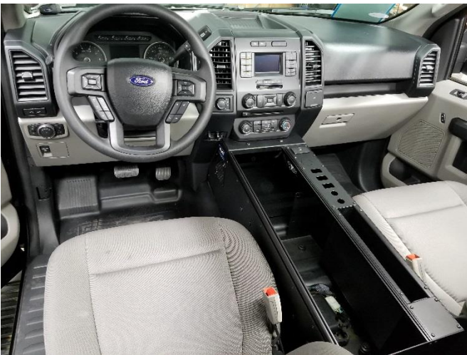
Main Housing installation is now complete. Install and wire equipment as desired.
