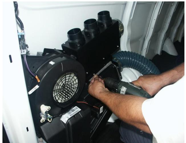
Connect Plenum (rectangle blower adaptor) to the O.E.M. blower ducts using #10 x 3/4" Sheet Metal Screws and #10 star washers.
