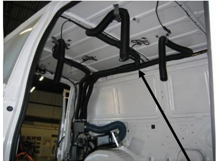
Attach the "Y" duct hose adaptor to the 8 foot front duct hose and connect both 4 foot hoses from "Y" to vents in driver and passenger side front ceiling. This will provide a total of four ceiling vents.
