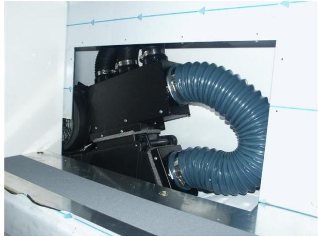
After Aluminum insert is installed and tested, attach cover plate to bench / wall to cover OEM Rear AC/Heat Unit using #10 Sheet metal screws.
