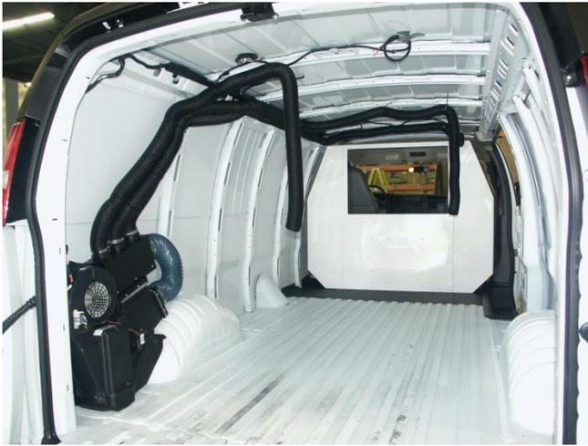
Route HVAC 2 1/2" blower hoses to the approximate locations with tape along ceiling where they will be installed into the ceiling after insert is installed. Mount hoses with wire ties at wall and ceiling corners only. Leave enough slack to reach hoses for permanent mounting.
