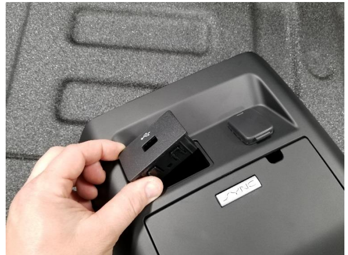
Remove OEM AUX module from dash and save to be reused.
