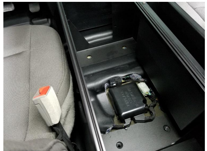
Slide console forward until the mounting brackets line up with the OEM mounting points in floor.
