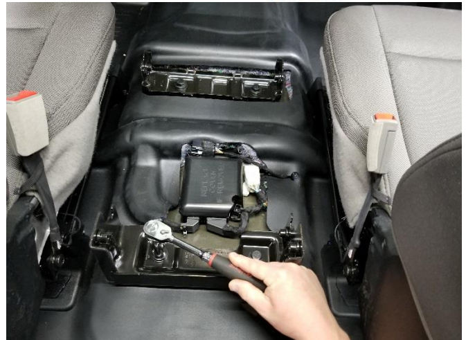
Unbolt factory bolts and save for later. 18mm socket
