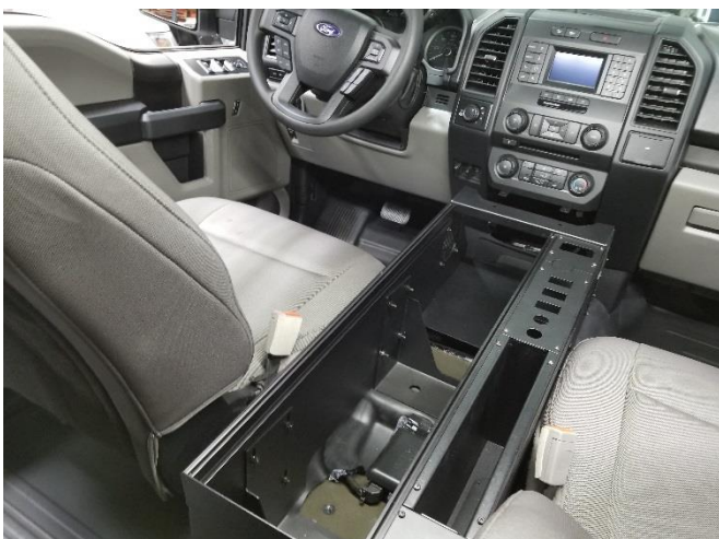
Place console with floor mount brackets into the vehicle. Shown with optional 3.3 wide panels and pocket.
