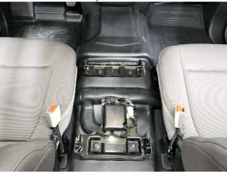
Remove factory center seat or mini console. Note: Seat belts (for center seat) must be left in vehicle and plugged back into OEM harness. Wire tie seat belts out of the way as desired.
