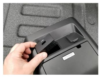
Remove OEM AUX module from dash and save to be reused.
