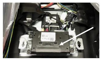
**NOTE:** Some vehicles include an OEM SmartLink / Telematics module mounted to transmission hump using the same bolts needed for the rear console bracket.
