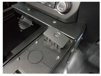
Install OEM AUX module into the console. Adaptor plate with #8 flat head screws provided for smaller Aux module. Blank plate provided if vehicle has no module for this location.
