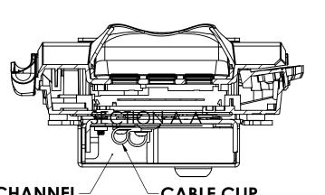
**CABLE ROUTING CHANNEL-**-CABLE CLIP **SECTION A-A**
