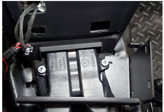
With cross supports detached, slide front mounting brackets under OEM studs from the sides.
