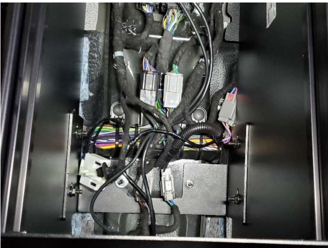
Attach housing to rear bracket with 1/4" x 3/4" carriage bolts and serrated nuts. Tighten all hardware.
