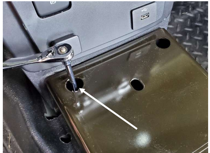
Remove OEM tunnel plate by removing rear nuts.
