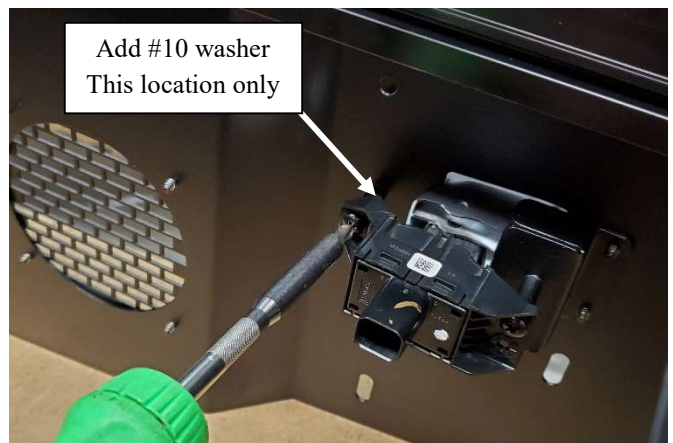
Install previously removed electronic emergency brake into side of console using supplied 10-32 x 3/8" machine screws. Add #10 flat washer for spacing between switch mount tab and threaded stud on console side panel.
