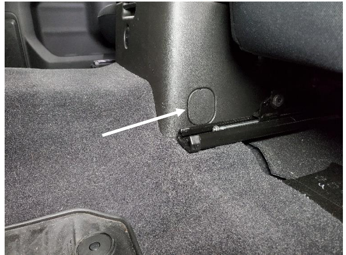
Remove covers on lower, forward sides of OEM center seat.
