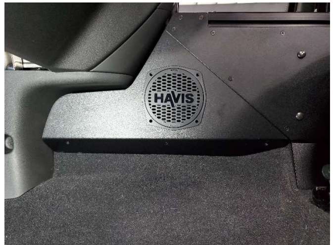
Snap speaker grills into side of console.
