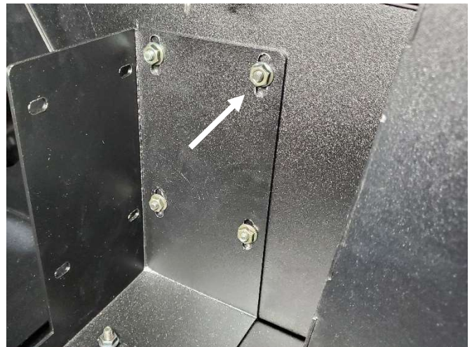
Attach passenger side console housing to mounting bracket with 1/4" x 3/4" carriage bolts and serrated nuts.
