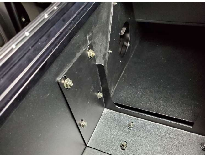
Attach driver side console housing to mounting bracket with 1/4" x 3/4" carriage bolts and serrated nuts.
