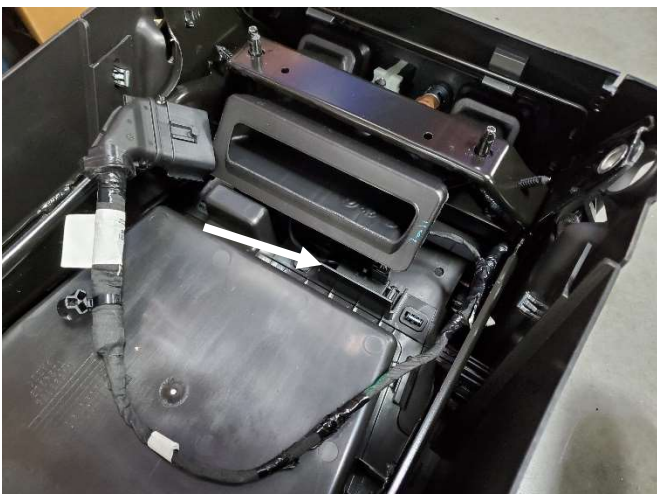
Remove wiring harness and proximity key module from under side of center seat. Plug harness back in and secure module to floor with wire tie.
