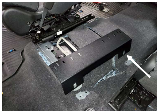
Attach floor mounting brackets using previously removed OEM hardware. Use 1/2" spacers at front between bracket and Trans hump.
