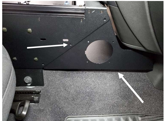
Attach side trim panel to console housing and equipment mounting plate using #8 flat head screws.
