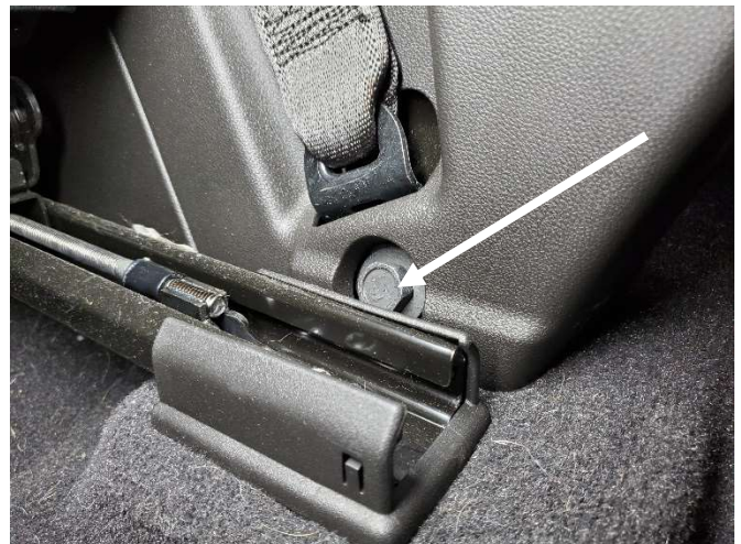
Temporarily remove front seats so you can access and remove the center seat rear bolts.
