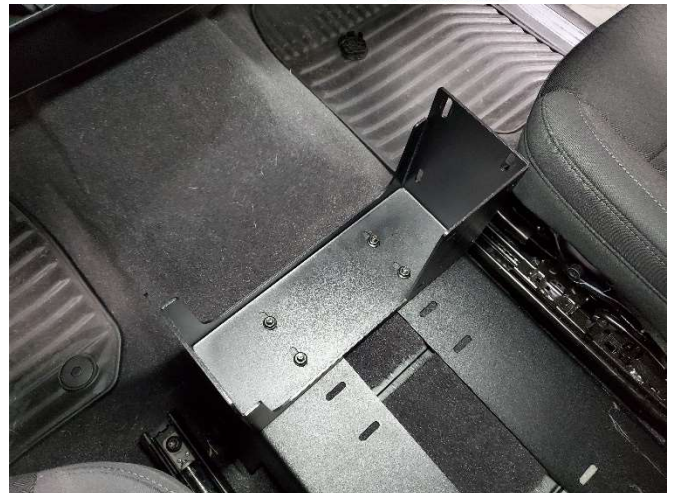
Place front mounting bracket on carriage bolts and attach with serrated nuts. Do not tighten yet.
