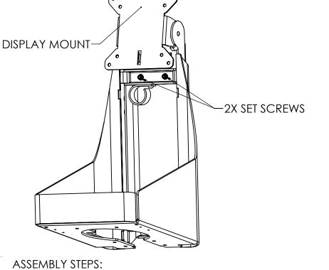
1. LOOSEN 2 SET SCREWS AND REMOVE DISPLAY MOUNT
