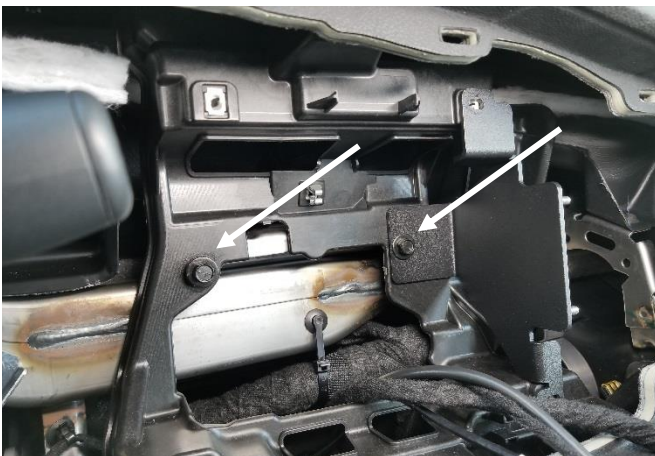
Temporarily remove two (2) OEM screws and attach support bracket with OEM screw as shown. 10mm socket.
