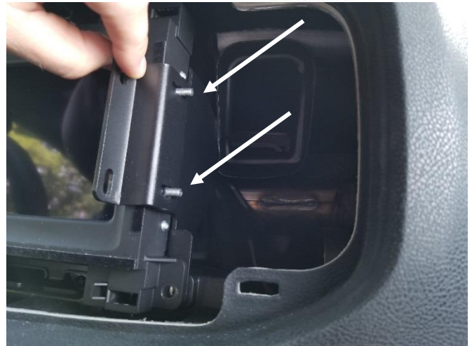
Attach side mounting brackets to the side support brackets using 10-32 nylock nuts and flat washers.
