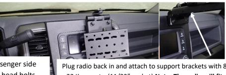
head bolts. ach bolt. Plug radio back in and attach to support brackets with 8-32 Keps nuts. (11/32" socket) Note: The radio will fit, but will be tight between the side support brackets.
