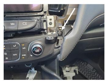
Remove OEM fastener and attach passenger side lower mounting bracket.
