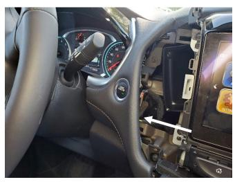
Unclip and pull back trim around push to start. *This does not need to be fully removed.*
