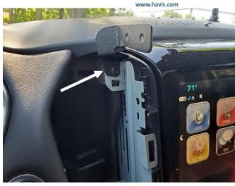
Remove OEM fastener and attach driver side upper mounting bracket.
