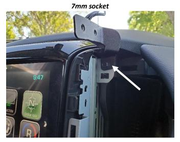
Remove OEM fastener and attach passenger side upper mounting bracket.
