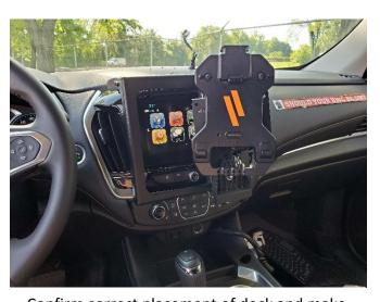
Confirm correct placement of dock and make sure rotation movement is smooth and latching works correctly.
