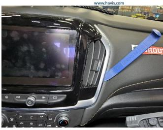
Carefully pry along sides of trim with a panel removal tool.
