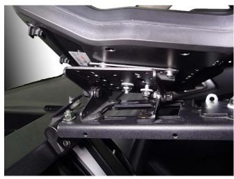
Determine desired position for your specific computer and attach to DMM swivel plate using 1/4"x 3/4" carriage bolts, PVC spacer, nylon washers, steel washers, and nylock nuts.
