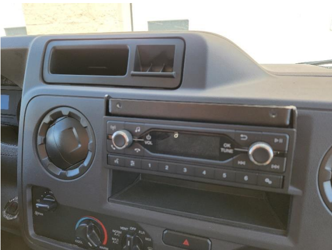
Plug radio harnesses back in and place radio in dash.
