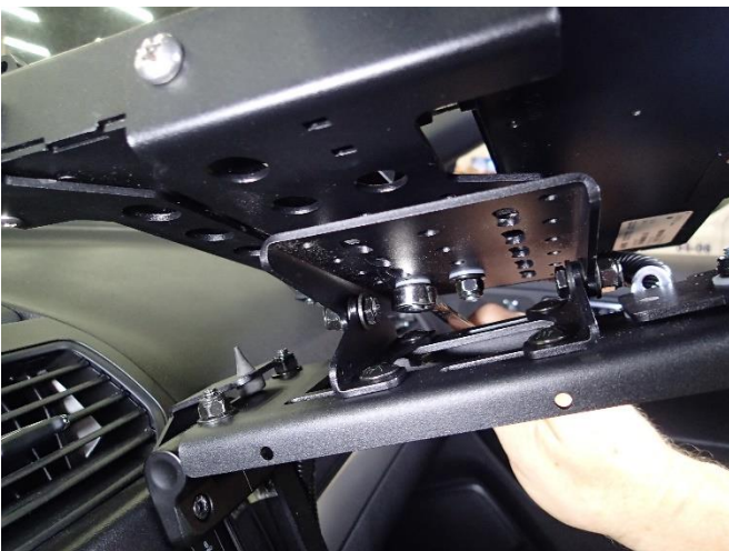
Determine desired position for your specific computer and attach to DMM swivel plate using 1/4" x 3/4" carriage bolts, PVC spacer, nylon washers, steel washers, and nylock nuts. Tighten so that the dock rotates smoothly.
