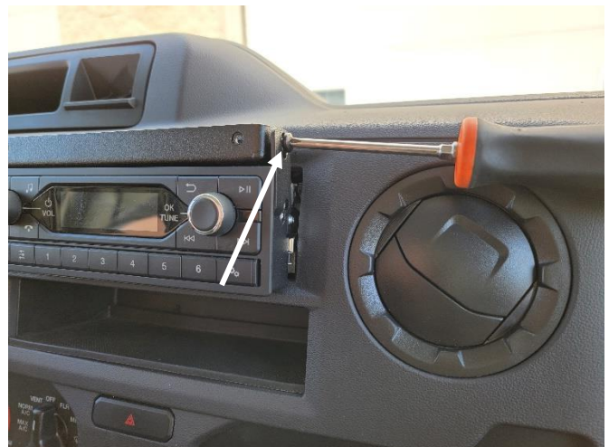
Attach radio U bracket to upper radio support bracket using 10-32 machine screws and washers.
