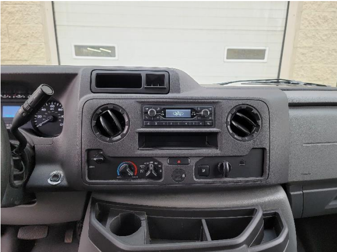
Using OEM radio removal tools, remove OEM radio from dash.
