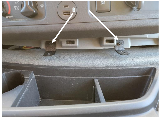
Pull dash trim away from dash to expose (2) 7mm head fasteners. Attach lower mounting tabs using OEM hardware.
