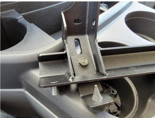
Loosely attach using 10-32 x 1/2" machine screw and keps nut. Place lower frame on lower mounting tabs and attach using 1/4" serrated nuts.
