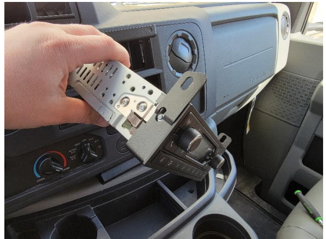
Slide up until snug on radio chassis.
