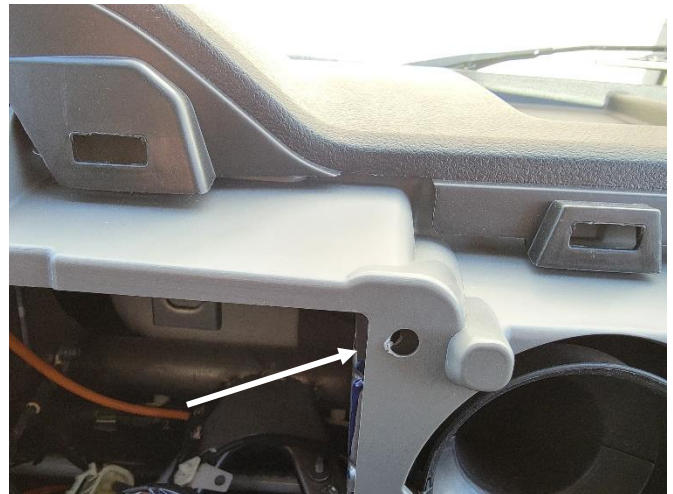
Slide clips into place ensuring they line up to opening.
