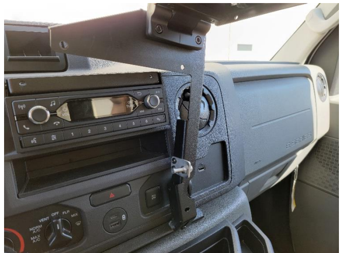
Place upper frame assembly onto lower frame.
