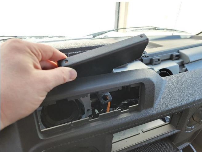
Slide upper radio support into dash, lining up with previously installed speed clips.
