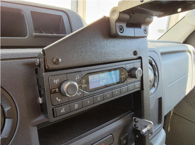
Attach upper frame assembly to upper radio support bracket using 10-32 x 1/2" machine screws.
