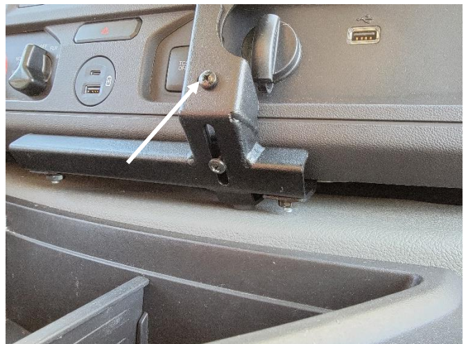
Attach upper and lower frame using 10-32 x 1/2" machine screws and keps nuts.
