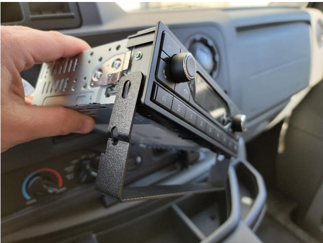
Place lower radio U bracket onto OEM radio.
