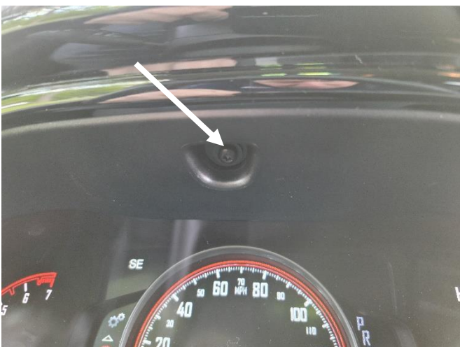
Remove T-20 Torx head fastener from upper, center of the instrument cluster.
