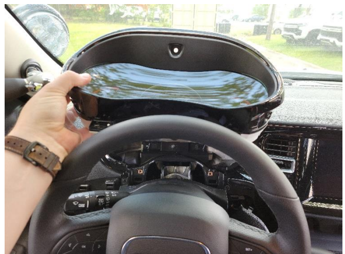
Remove instrument cluster. Cluster does not need to be unplugged. It can be set aside next to steering wheel.
