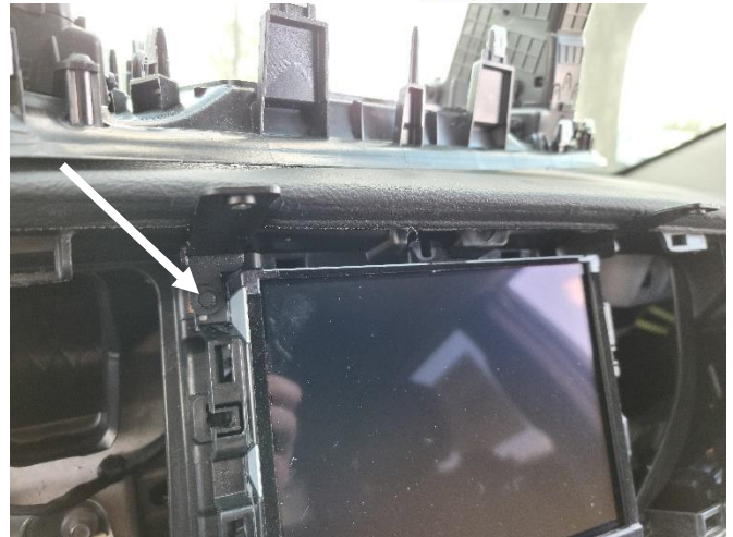
Remove 7mm head fastener from upper corner of radio and install DS upper mounting tab using OEM fastener.
