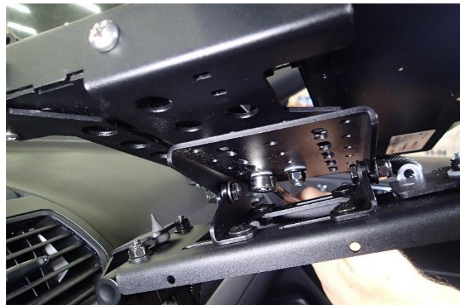
Determine desired position for your specific computer and attach to DMM swivel plate using 1/4"x 3/4" carriage bolts, PVC spacer, nylon washers, steel washers, and nylock nuts. Tighten so that the dock rotates smoothly.
