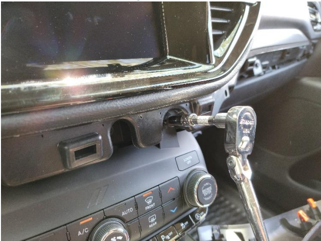
Remove 7mm head fastener from lower trim.
