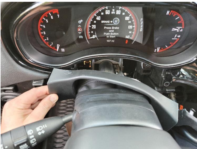
Remove trim around lower instrument cluster.
