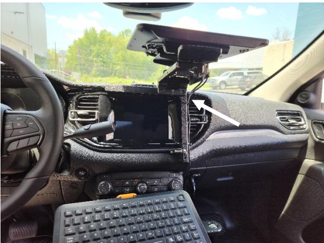
Route wiring as needed along the side of the DMM flip up frame using wire tie holes as shown. Test up / down and side to side motion to confirm wires have adequate slack and strain relief.
