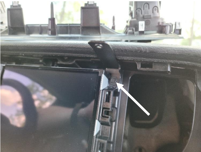
Remove 7mm head fastener from upper corner of radio and install PS upper mounting tab using OEM fastener.
