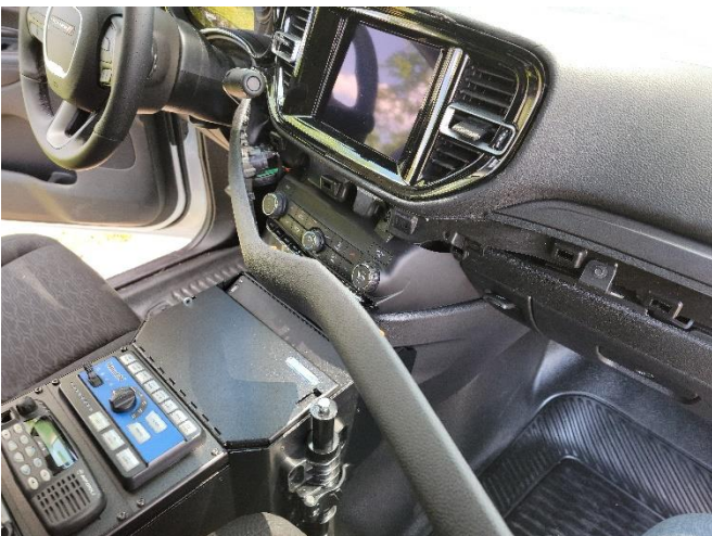
Continue removing trim along dash and set aside. Push to start does not need to be unplugged.
