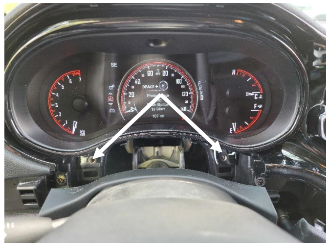
Remove (2) T-20 Torx head fasteners from instrument cluster.
