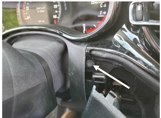
Remove 7mm head fastener from center trim.
