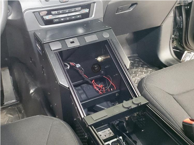
Slide console housing over floor mounting brackets and push tight to dash.
