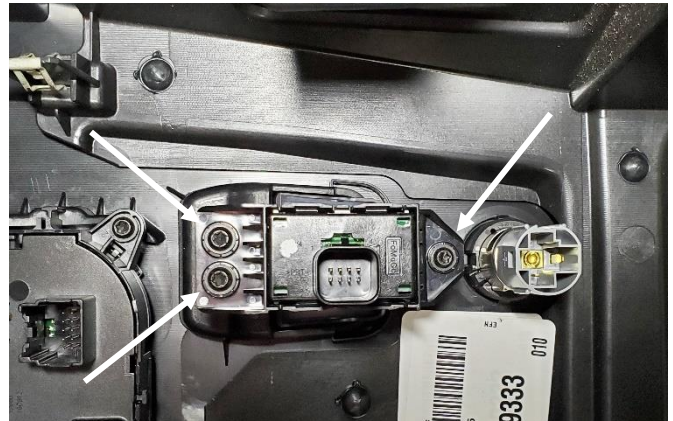
Remove electronic parking brake, 12 v socket and USB retaining bracket. (T-20 fasteners) If vehicle is equipped with rear HVAC, the controller will be removed at this time.
