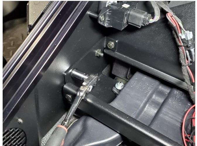
Attach housing to brackets with 1/4" x 3/4" carriage bolts and serrated nuts.
