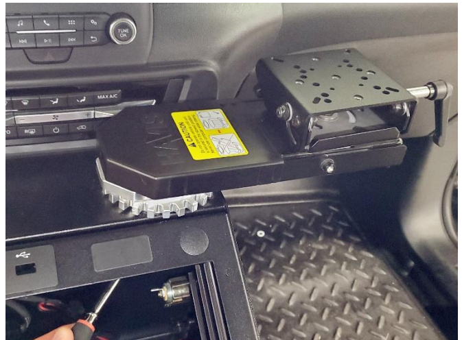
If a top motion device is used. Attach to top console plate prior to control head faceplates.
