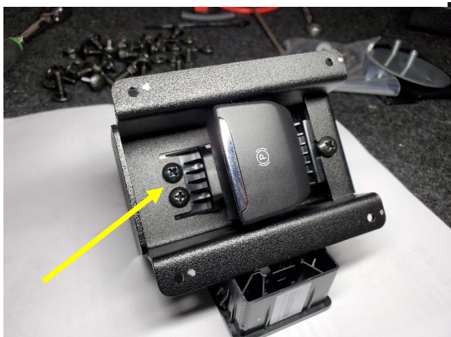
Install previously removed parking brake switch into supplied relocation bracket. The angled section with two holes goes under the lip of the bracket.
