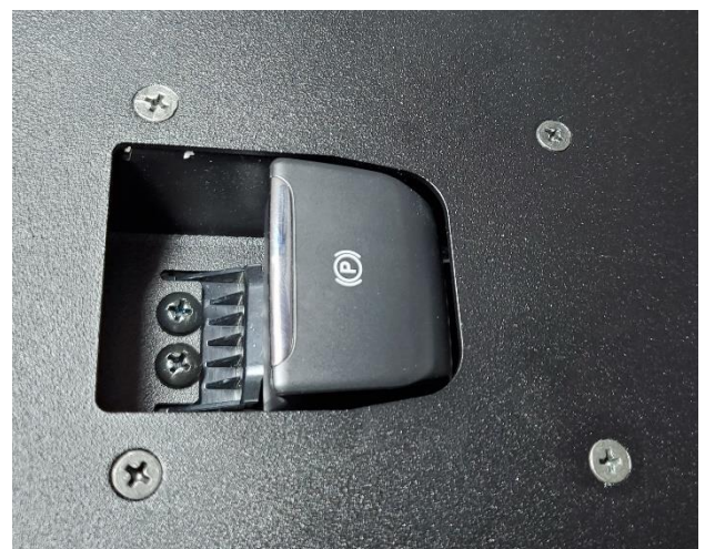
Attach parking brake bracket with switch to console using (4) #8 x 1/4" flat head screws.
