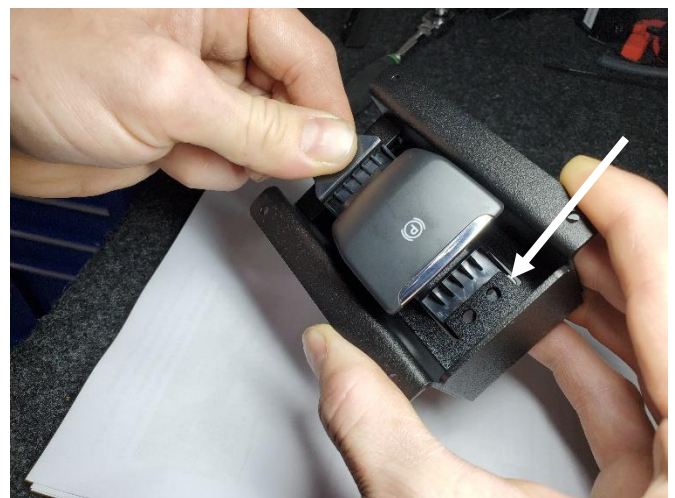
Install previously removed parking brake switch into supplied relocation bracket. Angle the section with the two holes under the lip of the bracket.
