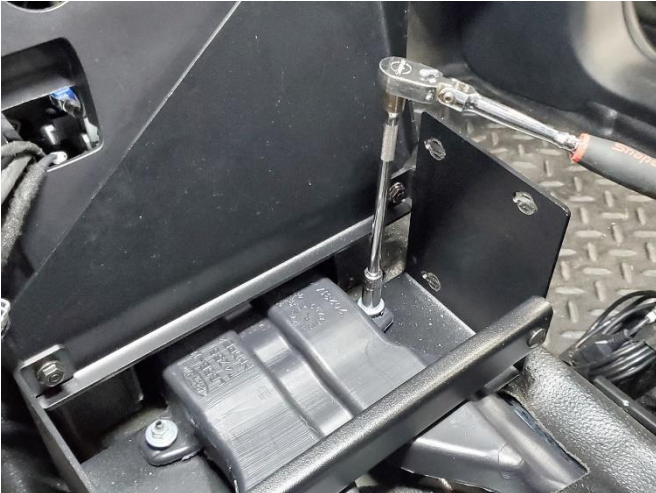
Retighten OEM ductwork nuts and bracket hardware.
