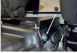
Place floor, mounting brackets over holes in floor and attach using M12 x 1.75 bolts and 7/16" flat washers. Note: You must use a 12mm x 1.75 tap to thread holes on PPV without OEM center seat or console.
