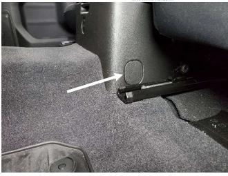
Remove covers on lower, front sides of OEM center seat.
