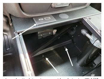
Loosely attach tray to support bracket using (2) 1/4" x 1/2" bolts, split lock washers, and flat washers.
