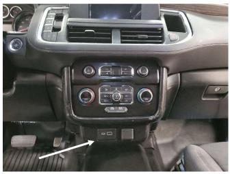
OEM aux panel must be removed from OEM lower dash.
