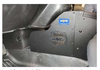
Attach forward side filler panels to console and equipment mounting tray using #8 x 3/8" Torx screws. Tighten all mount hardware Install OEM 120 volt socket into passenger side panel.
