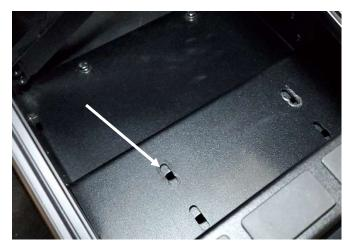
Loosely attach forward support bracket to floor brackets with 1/4" x 3/4" carriage bolts and serrated nuts.
