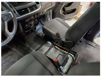
We highly recommend bolting seats back in after console is installed. This makes installation much easier.
