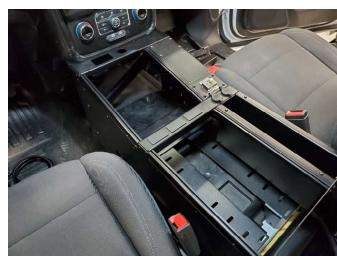
Place console housing with forward support bracket onto floor mounting brackets and slide housing toward dash.
