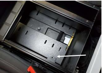
Loosely attach rear console housing and lower rear trim panel to floor brackets with 1/4" x 3/4" carriage bolts and serrated nuts.
