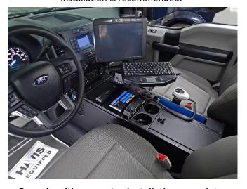
Console with computer installation complete.
