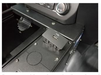
Install OEM AUX module into the console. Adaptor plate with #8 flat head screws provided for smaller Aux module.
