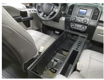
Place console with floor mount brackets into the vehicle. Shown with optional 3.3 wide panels and pocket.
