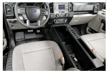
Main Housing installation is now complete. Install and wire equipment as desired.
