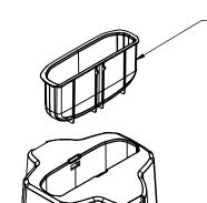
REMOVE INSERT IF USING RUGGED BOOT ON TC53/TC58
