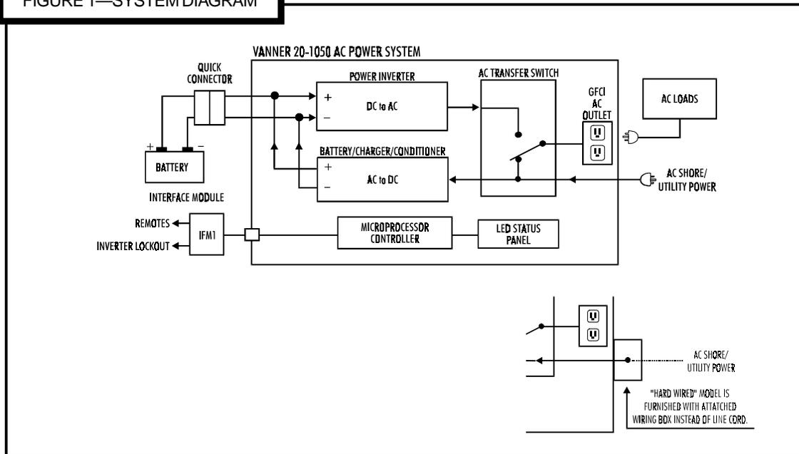
The charger automatically enters the Ready/Maintenance mode, maintaining the battery's proper voltage of 13.2 VDC for flooded batteries or 13.6 VDC for gel batteries. This Ready/Maintenance mode is designed to eliminate gassing (overcharging), helping to extend the life of the battery.
