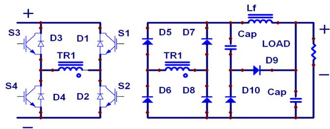
Fig. 11 Improved phase shift control topology
