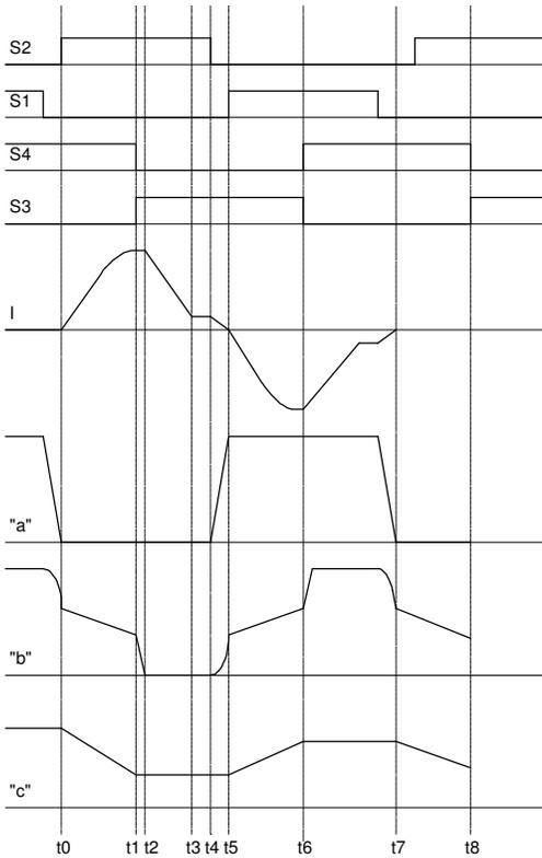
Fig. 2 Theoretical waveforms of the converter
