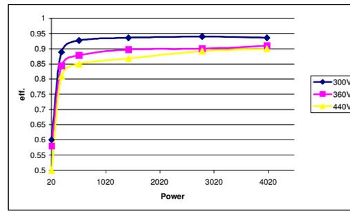
Fig. 8 Efficiency vs load
