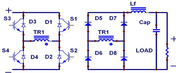
Fig. 10 Standard phase shift control topology
