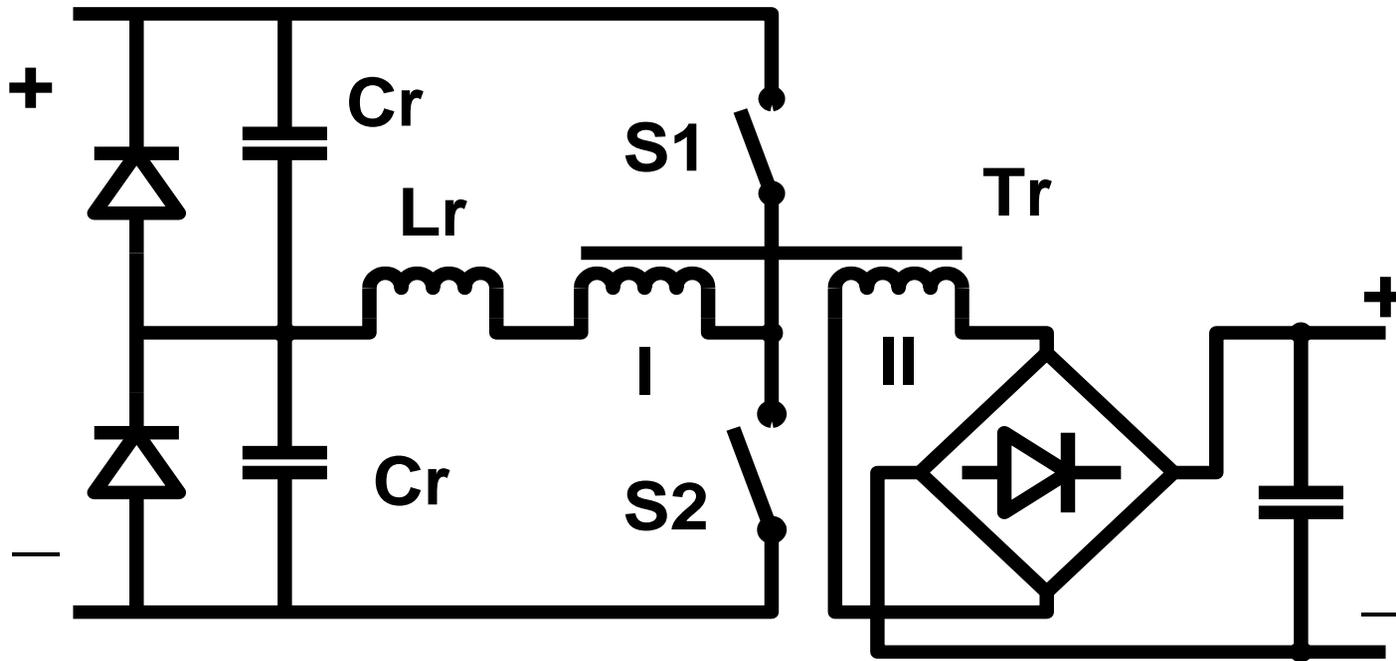
**Resonant topologies with clamp diodes provide passive power limiting.**
