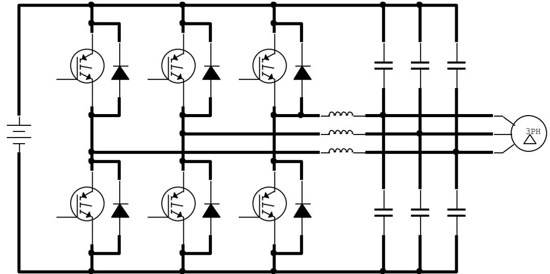
**System with a filter has higher efficiency under light load,**
