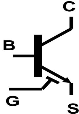
**ESBT symbol and equivalent circuit, cascade connection**
