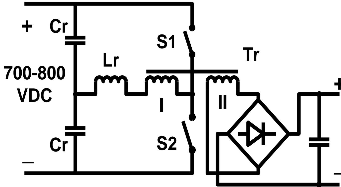
**Commutation Frequency-80kHz Current via Primary winding of transformer is sinusoidal with peak 60A and duty cycle 90-95%**
