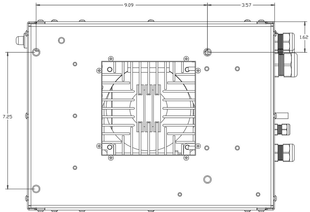
**Figure 2 – MPG Bottom View and Hole Locations**
