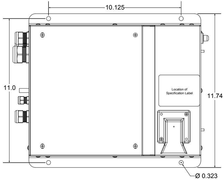
**Figure 6 - Shelf Mount Top View and Hole Locations**
