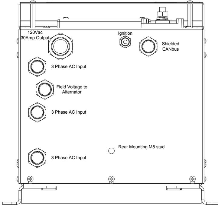
**Figure 8 – MPG Shelf Mount Rear View**
