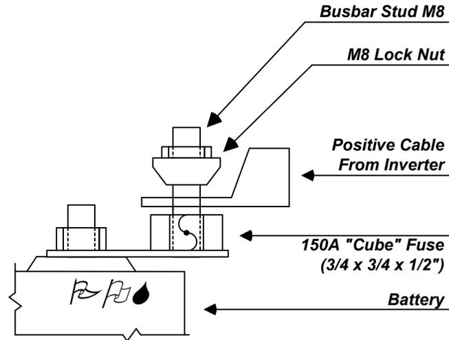
Figure 13 - Cube Fuse Wiring
