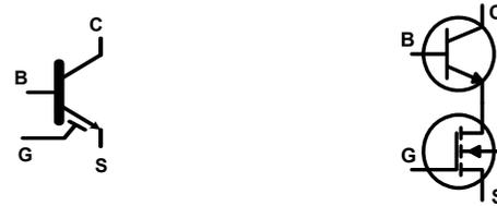
Fig.10 ESBT symbol and equivalent circuit, cascade connection
