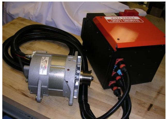
Figure 1. A 4kW Dynamic inverter system for a work truck
